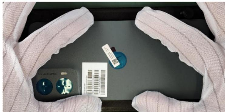
Step 5, Use fingers to press the surrounding Inlay Adhesive 3 times to activate it as shown and peel off the liner.
