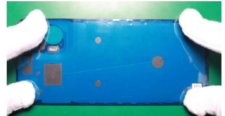
Step 6, Use fingers to place the Battery Cover on the phone as shown.
