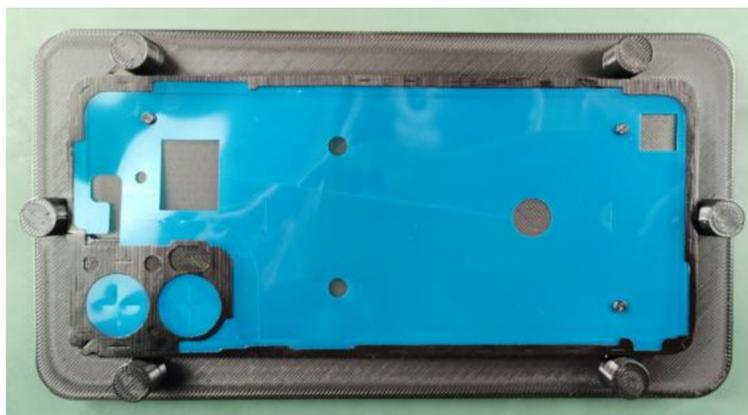
Step 3, Use hand put inlay in fixture. Locate the inlay with fixture big poles and align inlay rear camera area with fixture big location pole,
